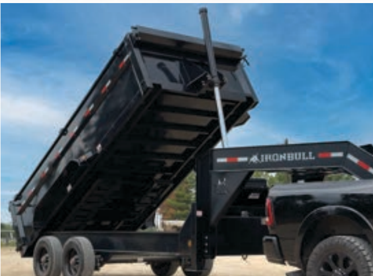
3 Stage Telescopic Cylinder (12 tons x 144")
